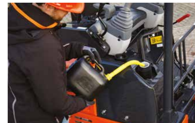
Sufficient space around the fuel tank opening for easy refuelling.
