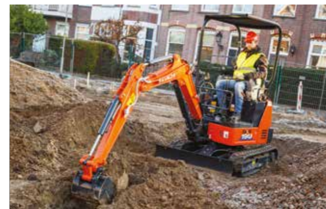
Expandable crawler tracks enhance versatility and stability.
